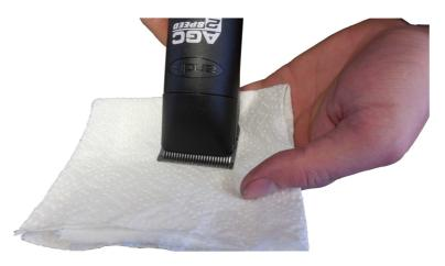
1. Oil the blade with 6 drops of oil as shown in the picture
