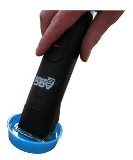
4. To clean the blade run in a bath of bladewash or white spirit. Then wipe off the excess.
